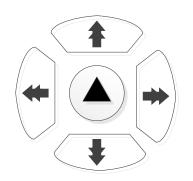
Press the center key repeatedly to change mode to Arrows control CAM/MON.
